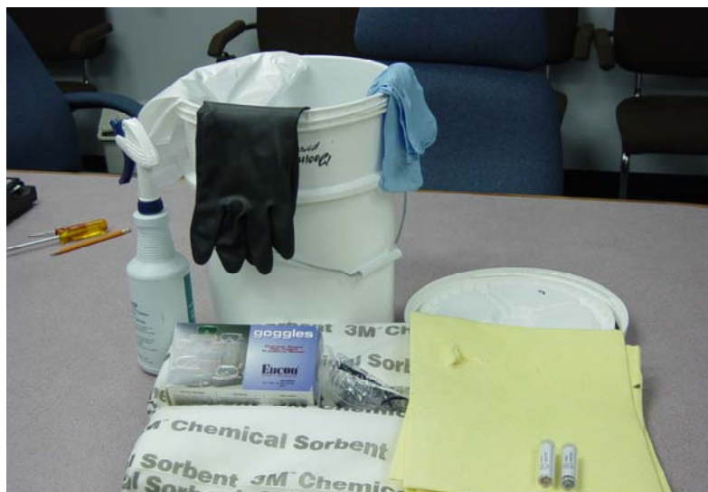
Figure 3: Generic spill kit. Kit includes absorbents, goggles, litmus, a neutralizer, gloves, and waste bags. The bucket can be used for lab packing.
